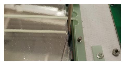
At least 1 mm gap at room temperature between G2P WLS bar and HPK SiPMs → it increases at cold (~2 mm).
