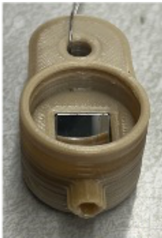
New single hole design of diffuser
