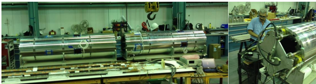
Fig. 4.7. Left: Two half-length yoke-shell subassemblies, ready to be joined. Right: hydraulic rig for pre-tensioning the yoke tie rods.
