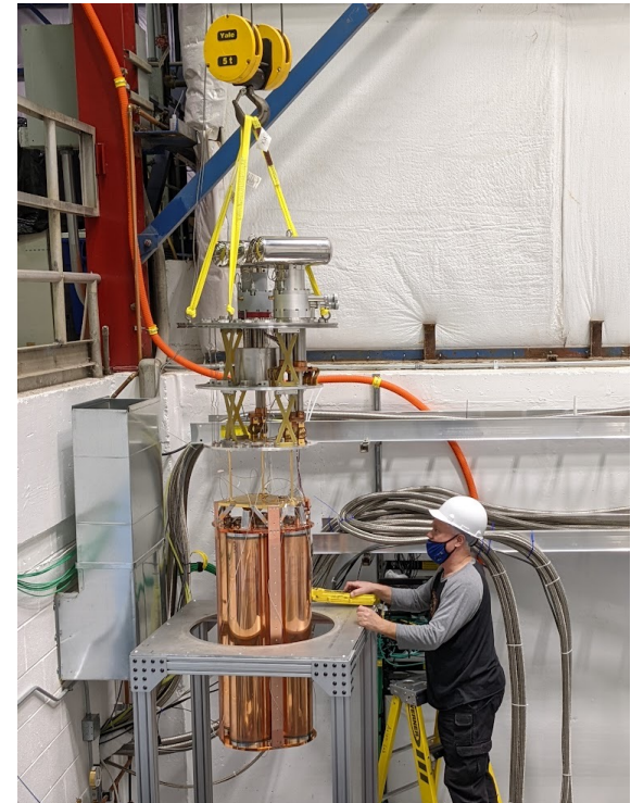
ADMX-G2 Resonator Testing in Fermilab's axion lab at SiDet
