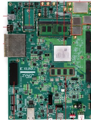
ZCU111: FPGA+ADC+DAC+ memory+interfaces
