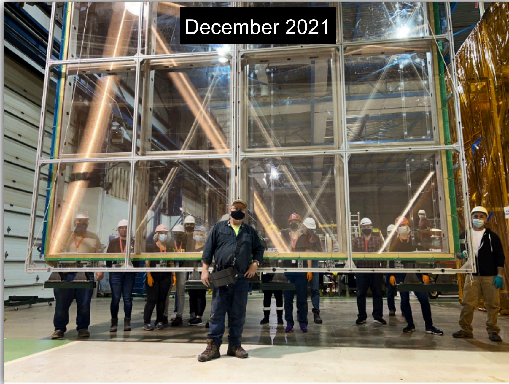
Installation of the EAST Anode plane
