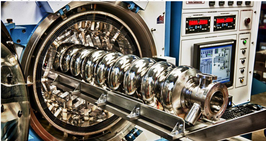
Figure 1: Nb SRF Cavities lined up and being tested with a magnetic field.
