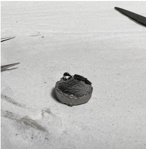
Figure 15: A Nb cavity cutout. Notice the highly raised edges, making incident radiation analysis difficult. Retrieved from SQMS.
