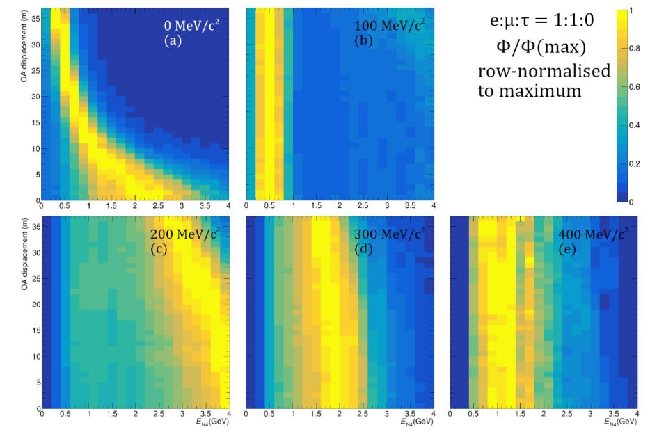
Flux shapes, using ND baseline 575m from origin @ beam angle = 5.8° downwards
