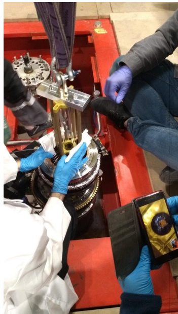
Lowering Torlon into P2 feedthrough
