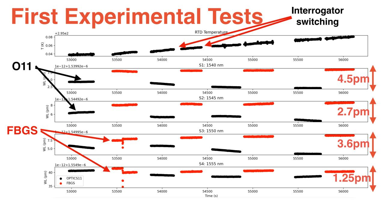
There exists a clear difference in the measurements taken using O11 and FBGS interrogators. O11 is more sensitive to changes than FBGS.
