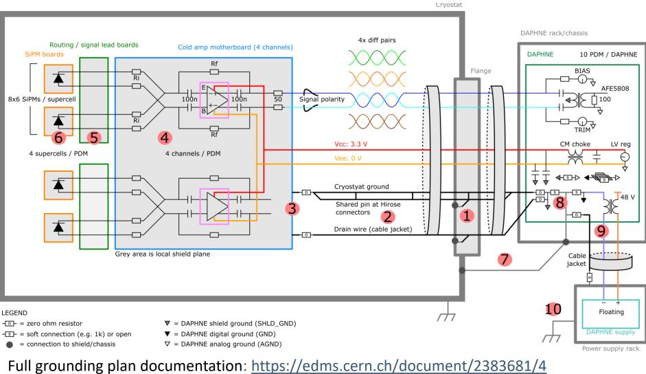
Full grounding plan documentation: <u>https://edms.cern.ch/document/2383681</u> (sytem is in a star-ground configuration with the hub at the cryostat flange) Cables: <u>https://edms.cern.ch/document/2383682/4</u>
