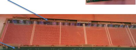
The motherboard hosting the cold amplifiers (one amp per supercell/channel, 4 per module)
