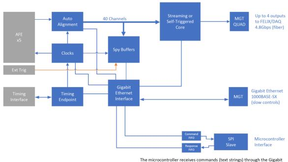
Ethernet interface. This replaces the microcontroller 100 Mbit Ethernet interface.
