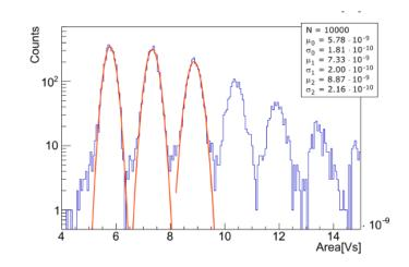
S/N = 8 at 45% PDE and 2000 p.e. dynamic range for both FBK and HPK SiPMs Power consumption: 0.7 mA/channel at 3.3 V, i.e. 2.4 mW/channel
