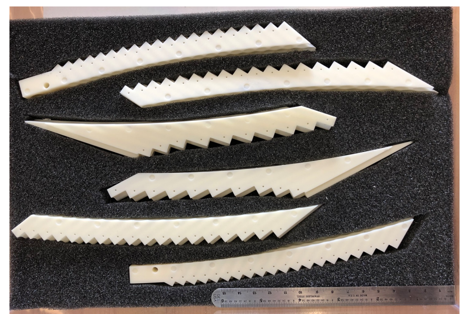
6 part Plastic Inner ring of Mu2e panels
