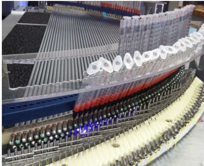
Epoxy holes allow for passive injection
