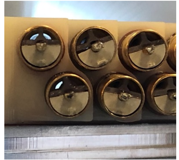
Light through termination gas openings
