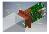
Redundant readout: For each crystal, two custom arrays ( $2 \times 3$  of  $6 \times 6$  mm2) large area UV-extended SiPM
