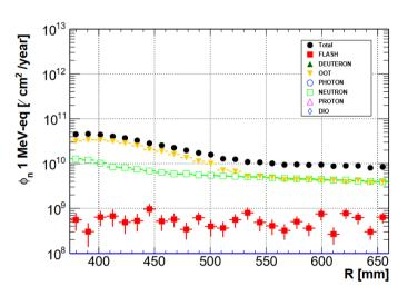
1MeV-eq n Fluence = simulated Fluence x3 Safety Factor, x3 yrs, x10 Mu2-II 5.4 X 10^12 n/cm^2
