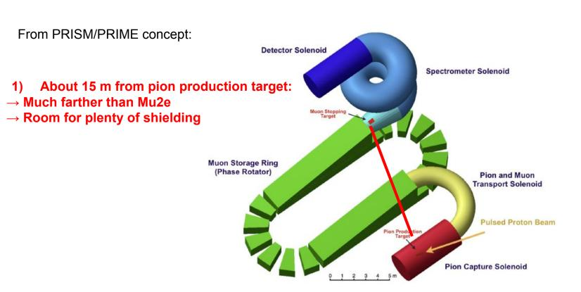
From PRISM/PRIME concept: **Detector Solenoid** Spectrometer Solenoid 2) Assuming we can shield the CRV from the muon stopping target, background rates in the CRV should be more manageable. Muon Storage Ring (Phase Rotator) Pion and Muon **Transport Solenoid Pulsed Proton Beam** Pion Capture Solenoid
