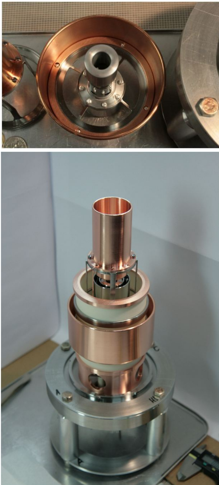
FIG. 6: Photographs of the 1-inch hollow electron gun. Top: detail of the cathode. Bottom: assembled gun.
