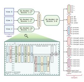
Separation of track- and shower-like energy deposits in ProtoDUNE-SP using a convolutional neural network
