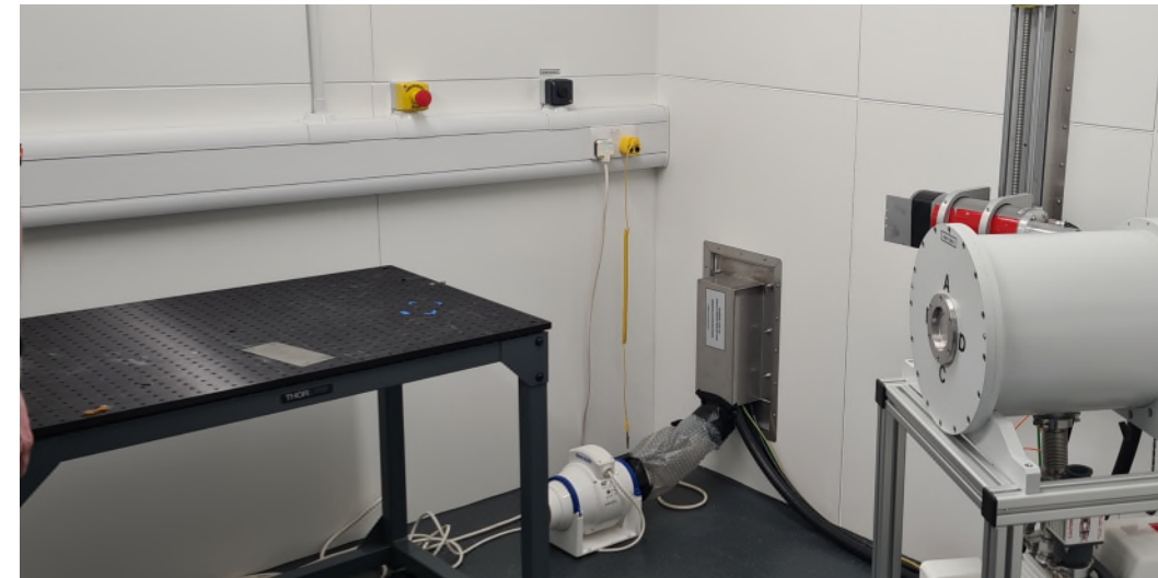
LBNF-UK Beam and Target System X-ray bay used. Continuous source is the red cylinder on the wall
