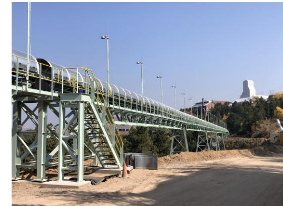
Rock conveyor system to move rock to Open Cut
