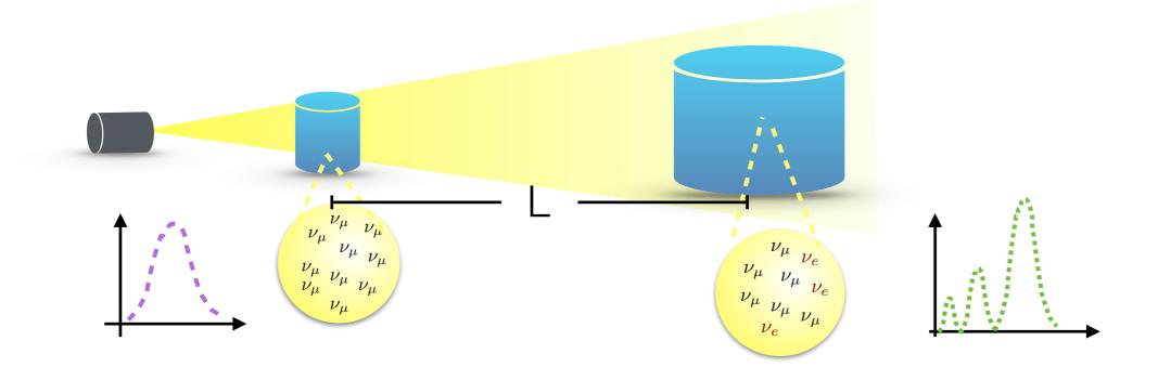
A precise determination of  $\sigma(E)$  is crucial to extract v oscillation parameters. Nuclear effects at near and far detector **do not** cancel
