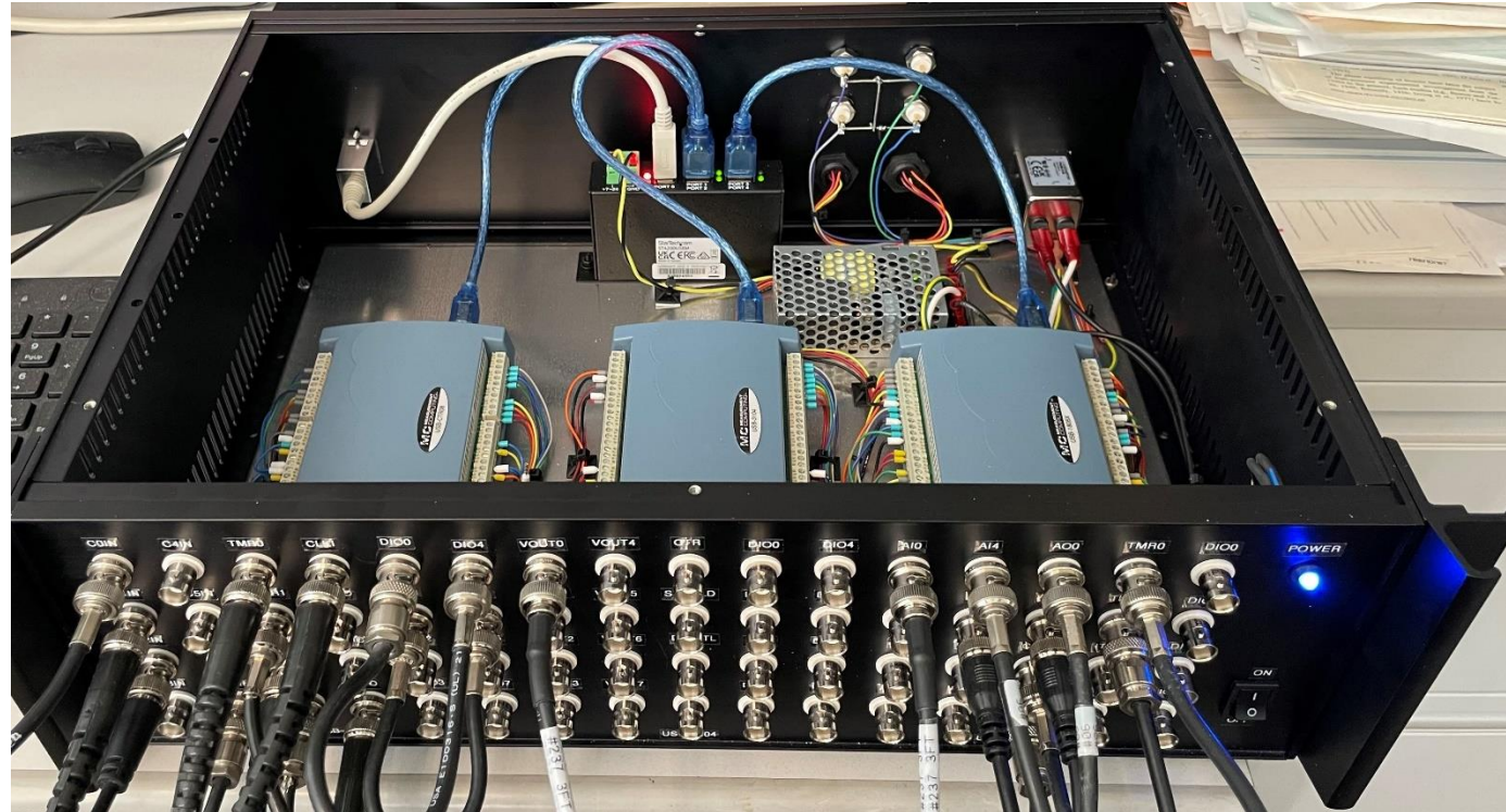
Our enclosure for USB-1808X, USB-3104, USB-CTR08, 68 BNC connectors, 2 encoders
