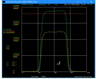
SPAD1 rate (green) changes when its horizontal position is changed linearly in time. LD current is  $\sim$ 30 µA. 1-Feb-23.
