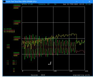
SPAD1/2 rates (green/red) vs stage position. LD current is  $\sim$ 30  $\mu$ A. 1-Feb-23.
