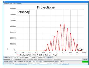
Projection on the horizontal axis. 31-Jan-23. LD current is 25.6 mA. Visibility changes dramatically from projection to projection.
