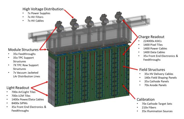
The image above shows one of the 7 rows of modules that make the ND-LAr detector with spares. Quantities provided in the diagram above are for 35 modules. The cryostat lid segment (in transparent grey) is outside of the ND-LAr Consortium scope.
