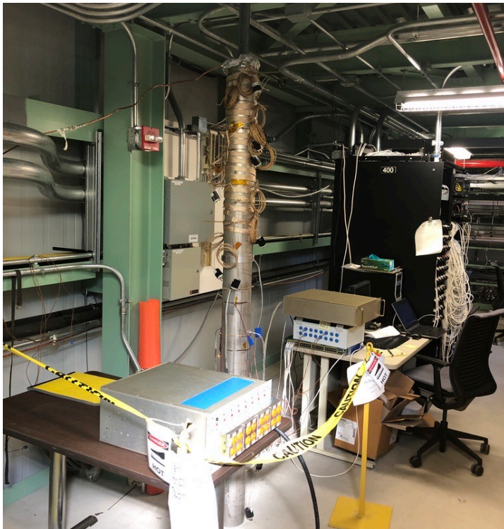
16-channel bake test setup.
