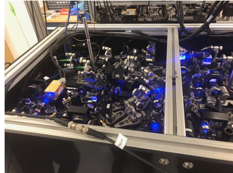
Optics in the top layer of the atom source.
