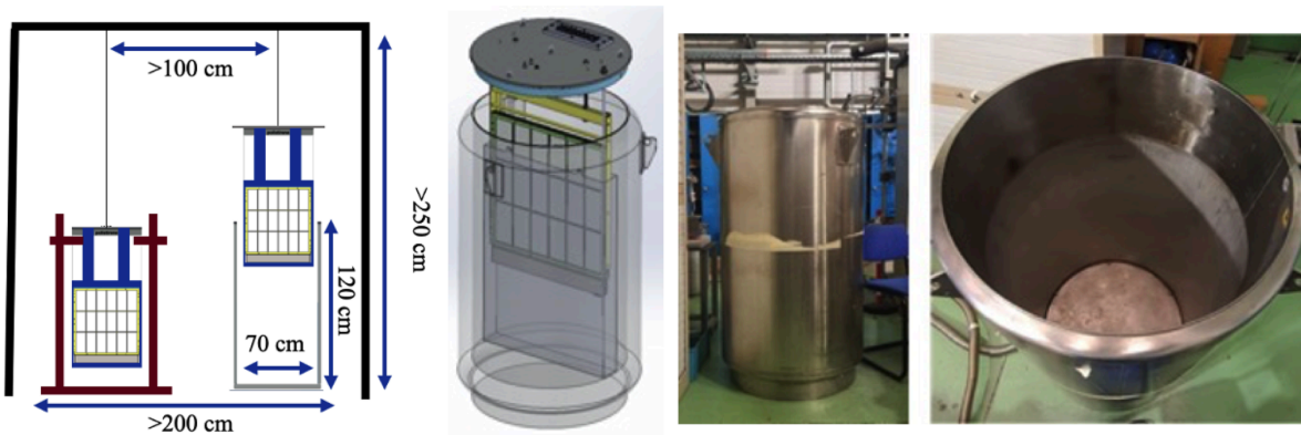
Figure 11. Cryo-test facility at CERN NP for full size XARAPUCA modules and read-out electronics tests.
