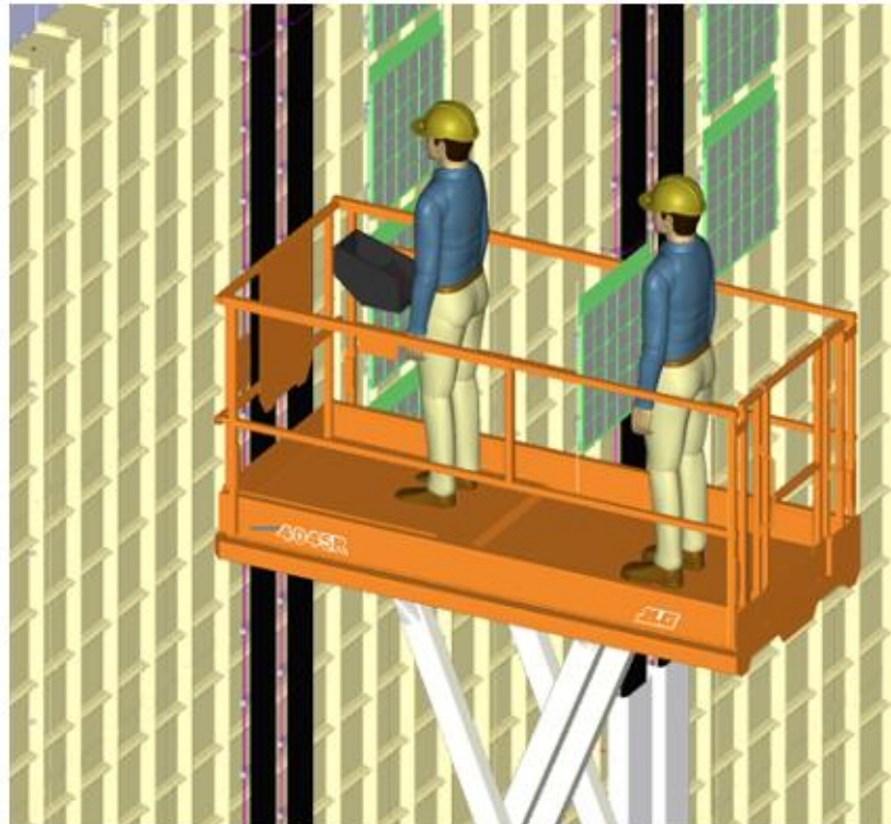
Figure 20. View of the top (4) Membrane-mount XA installation.
