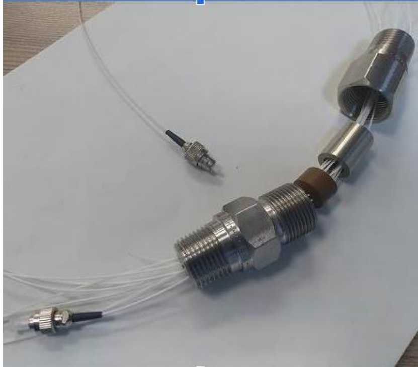
Figure 21. Cathode-mounted XA feedthrough for (8) SoF/PoF fibers before compression fit.
