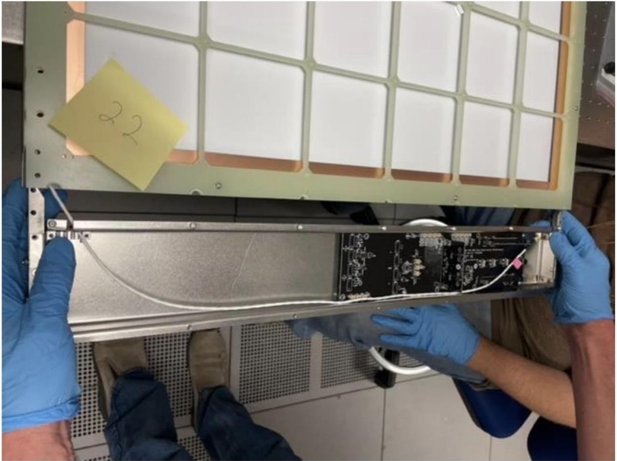
Figure 8. Electronics box kit attachment to the XA frame.
