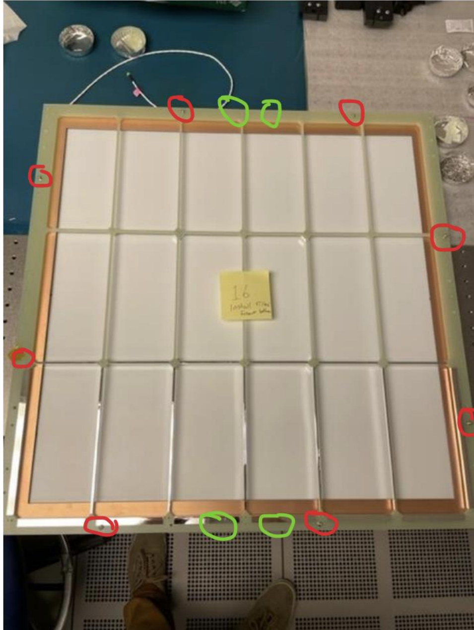
Figure 7. Top subframe fastener pattern of M3 (red) and M4 (green) screws.
