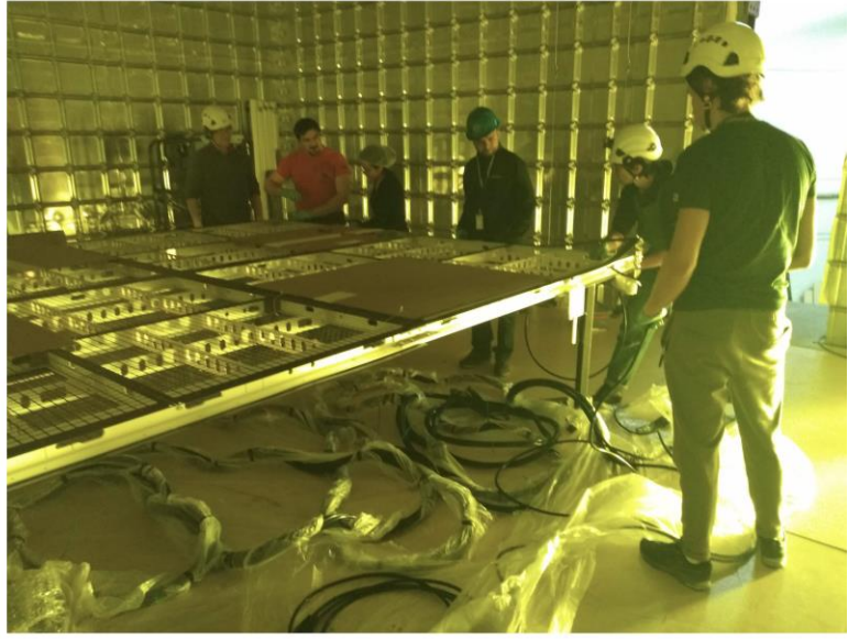
Figure 27. Fiber bundle moved to cathode at <math><2\text{m}</math> working height for routing on cathode.
