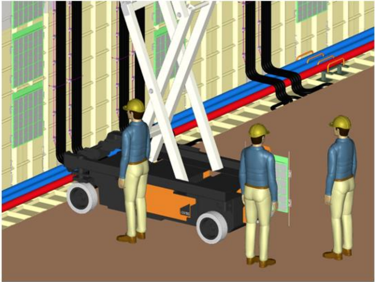
Figure 18. View of the cable/fiber dressing down to the floor of the cryostat.
