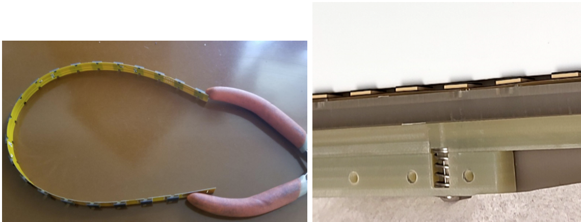
Figure 1.10: 20 SiPMs mounted to flexible PCB (left). Flexible PCB positioned against a dummy WLS plate (white block) with spring-loaded dynamic mount (right).
