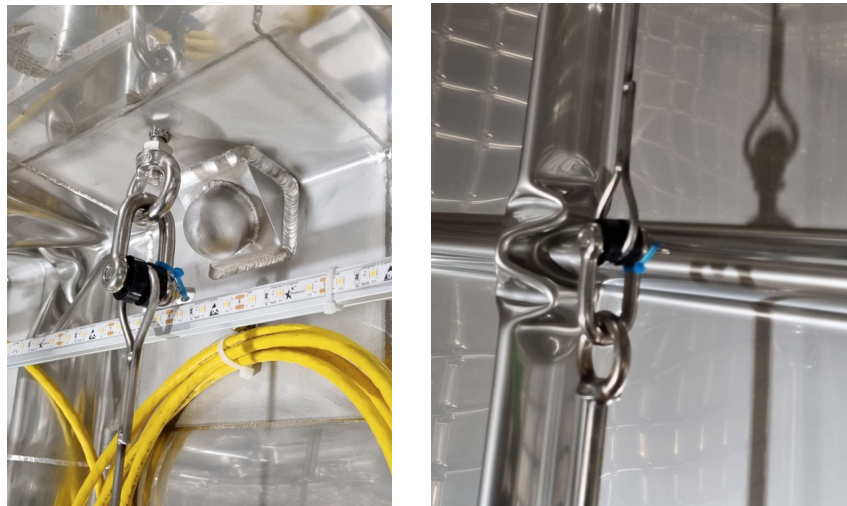
Figure 32. Left: anchoring one of the suspension lines to the top of the cryostat. Right: the connection between the top and middle sections of the suspension line. The middle section has a larger diameter to reduce the electric field at the surface since this section is closer to the cathode.
