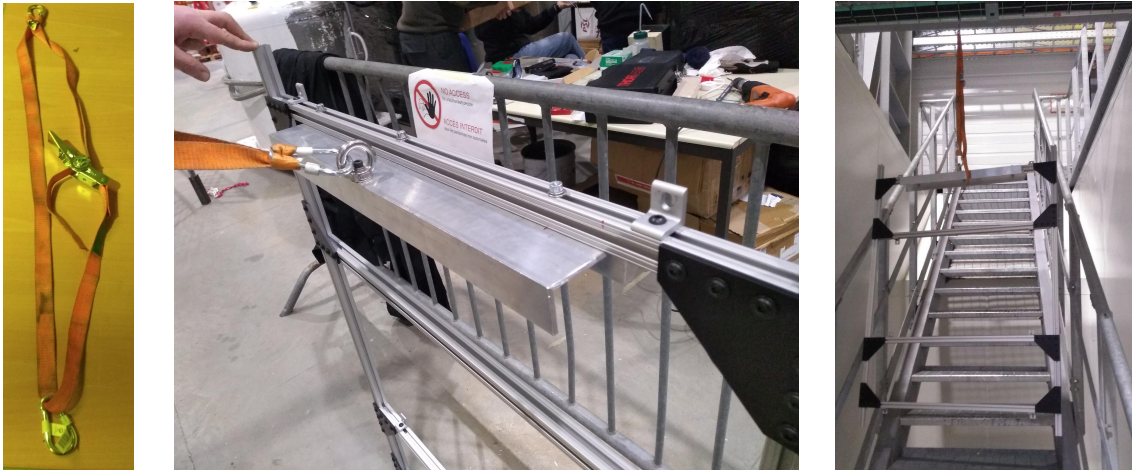
Figure 37. Left: View of the safety rope. Center: Detail of the steel ledge added to the support frame. Right: The safety rope holding the support frame.
