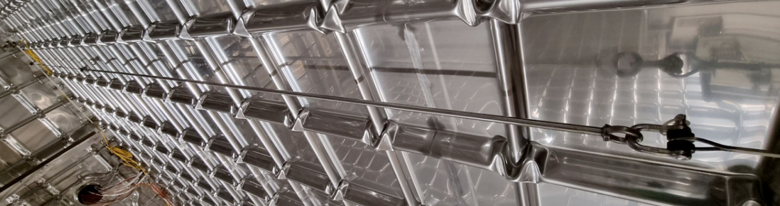
Figure 28. One of the two stainless steel suspension lines installed in each of the two short field cage walls.
