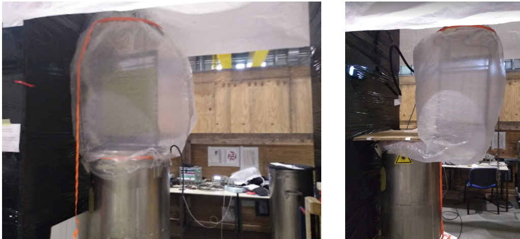
Figure 23. Left: plastic tent surrounding the XA with GN2 flashing. Right: plastic tent with XA displaced from dewar vertical to avoid cold gases that would slow down the warmup process.
