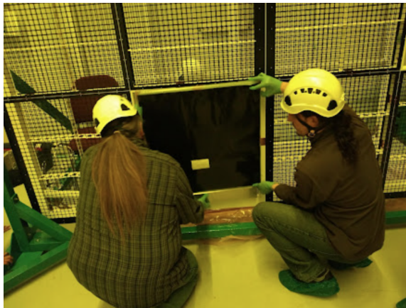
Figure 43: Installation of cathode modules with first cathode on cart wall
