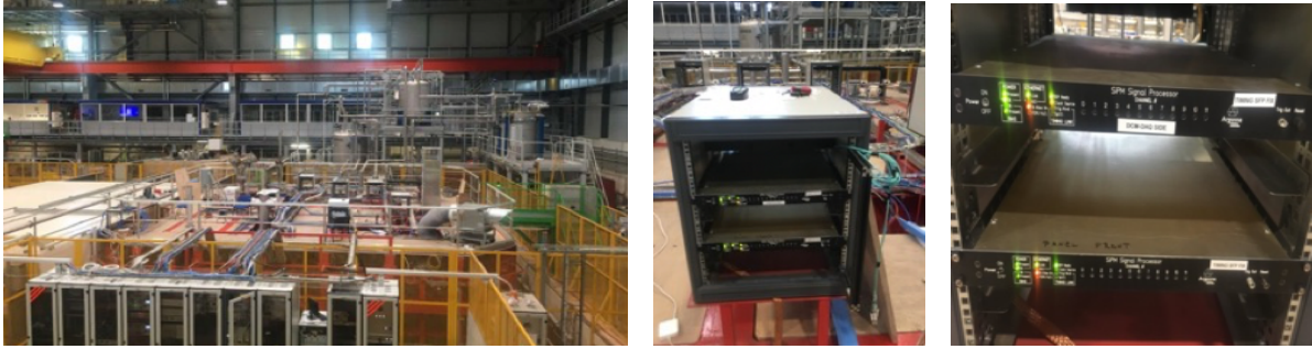
Figure 59. Left: ProtoDUNE-SP-II Cryostat at CERN with electronic racks at the top. Middle and right: PDS electronics calibration modules (5-channel prototype module and 12-channel module for ProtoDUNE-SP-II) tested and integrated with timing and DAQ system at CERN.
