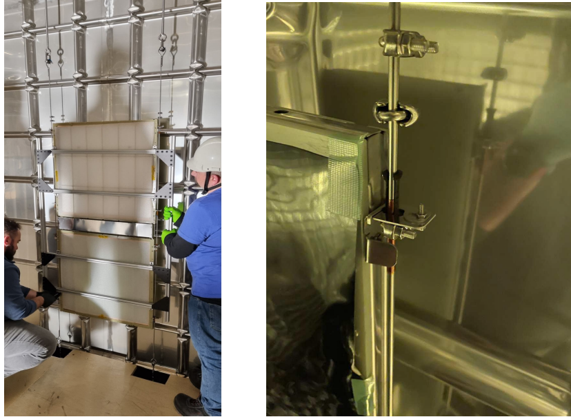
Figure 35. Left: Picture of the installation of the X-ARAPUCA modules in the bottom part of the membrane. Right: Detail of the metallic holders resting on the wire rope clamps.
