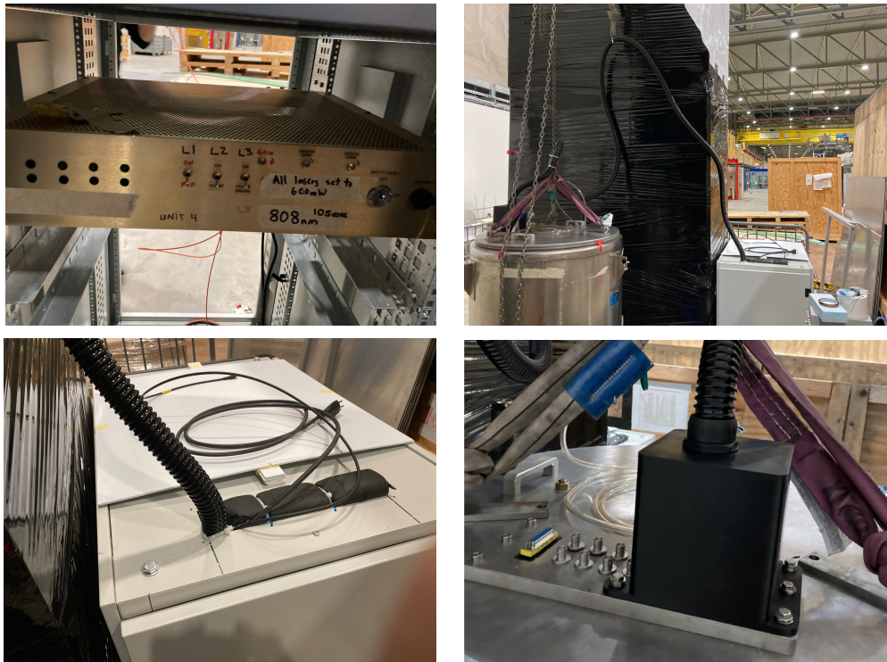
Figure 25. Top-left: the high-power laser case, located inside the mini-rack. Top-right: general view of the dewar, the mini-rack and the corrugated black tube used to protect the fibers in its path from the mini-rack to the dewar lid. Bottom-left: Detail of the corrugated black tube entering in the mini-rack. Bottom-right: 3D printed box used as strain relief for fibers connected to the dewar lid FC-FC feedthrough, also serving a protection against laser light leakage.
