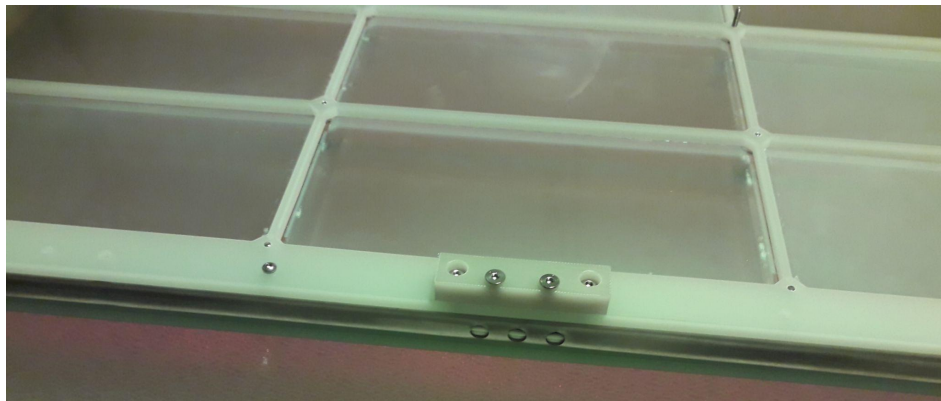
Figure 41. Detail of G10 block attached to cathode module C2. The two center holes are for cathode frame attachment.
