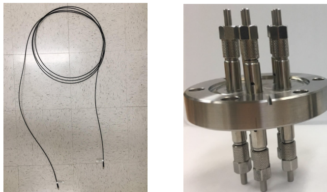
Figure 60. Left: Warm Optical Fiber. Right: Optical feedthrough units for ProtoDUNE. The feedthrough is attached to the optical flange to transport UV light from the Calibration Module to the diffuse fiber ends, via the optical fiber system.
