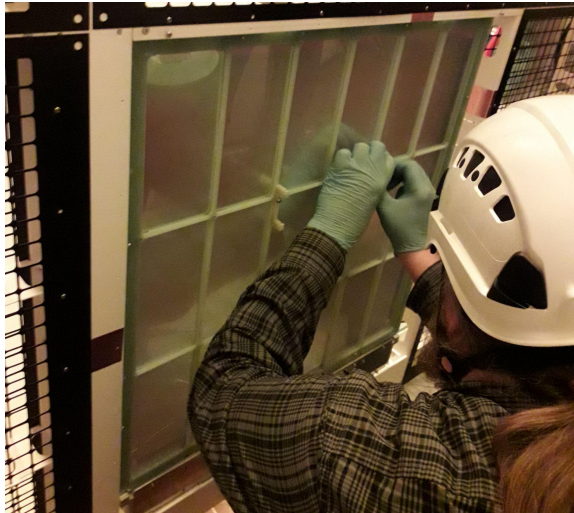
Figure 44. Left: Placement of the mesh support brackets (4 per side per module). Right: the cathode module and conductive mesh are in position.
