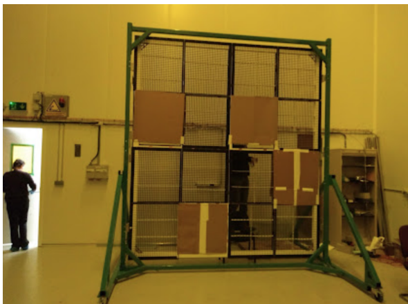
Figure 45. Left. All four cathode modules installed and protected with cardboard panels. Right: Inserting the first cathode on NP02 cryostat
