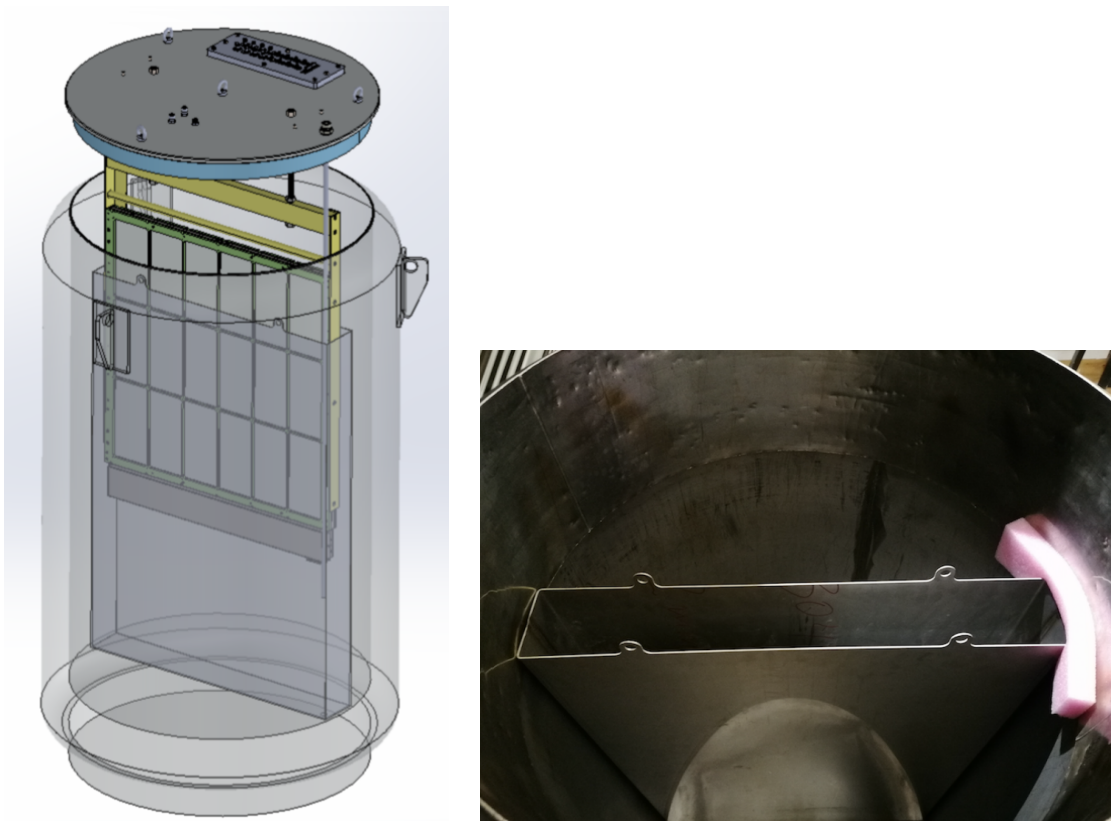
Figure 21. Left: 3D model of some of the elements of the testing setup, the open dewar, the inner box, the lid, the XA and its support. Right: the inner box.
