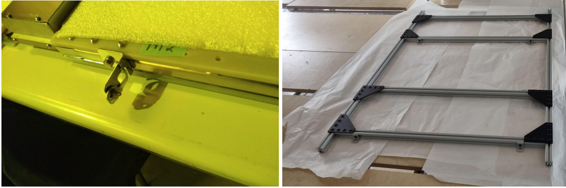
Figure 34. Left: metal holder installed on the membrane X-ARAPUCA. It has a scissor-like security closing tightened with a screw to attach to the stainless-steel line. Right: transport and installation support frame for two membrane modules.
