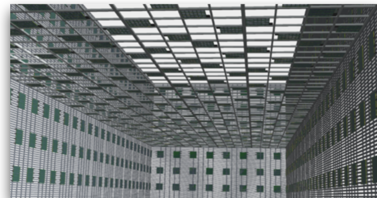
The \sim 4\pi PDS Concept with Cathode and FieldCage Coverage
