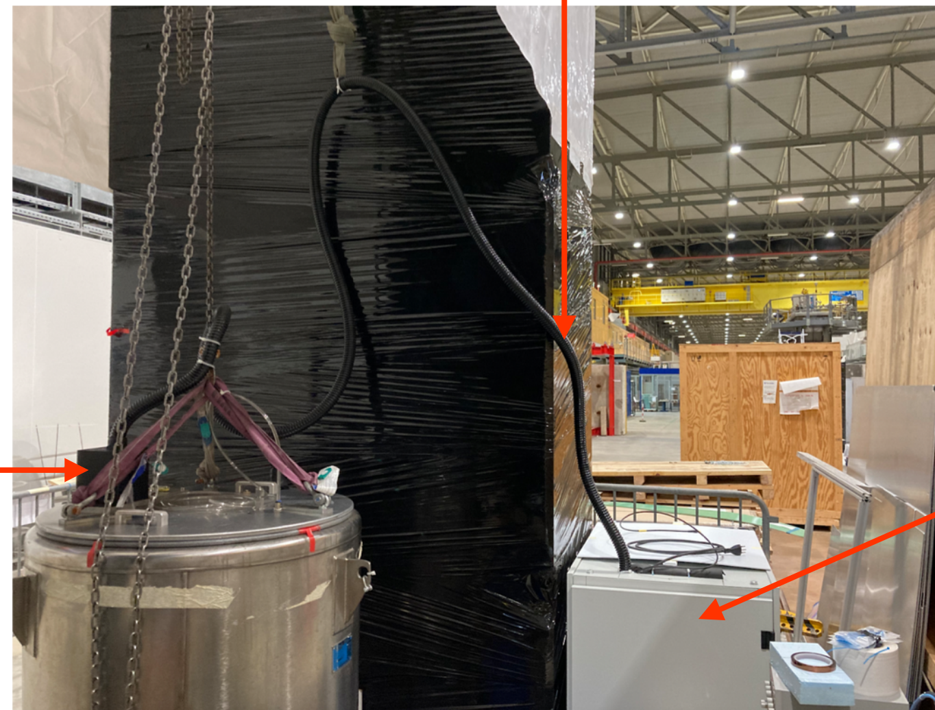
corrugated back tube from dewar to mini-rack
