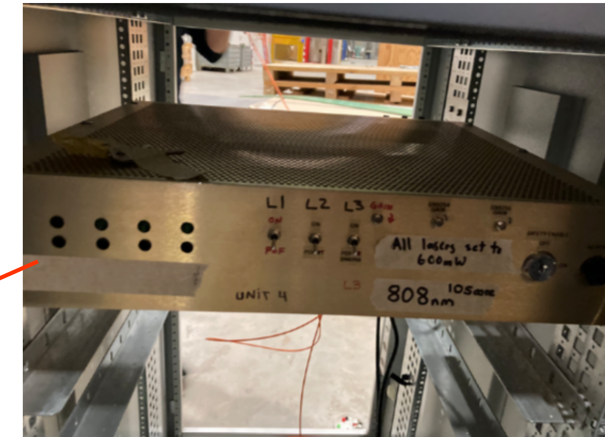
class-4 laser inside mini-rack
