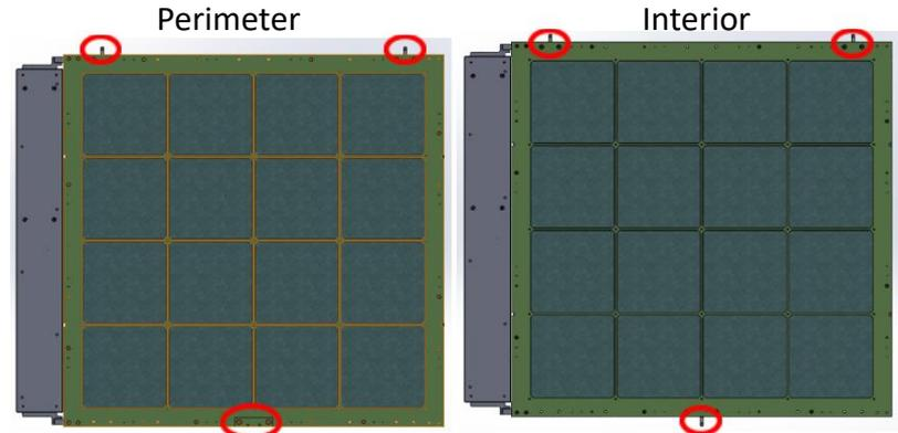
Figure 3: Perimeter Cathode Module Mounting Points (Left), Interior Cathode Module Mounting Points (Right)
