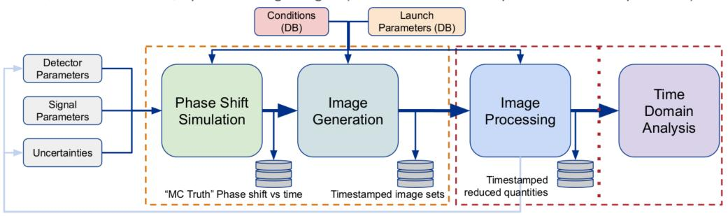
**Production analysis:** starting from the images, fit the patterns and extract a phase shift ("image processing"). Should be able to run on both simulation and real data with minor user input. These algorithms should be used in both Online and Offline processing
