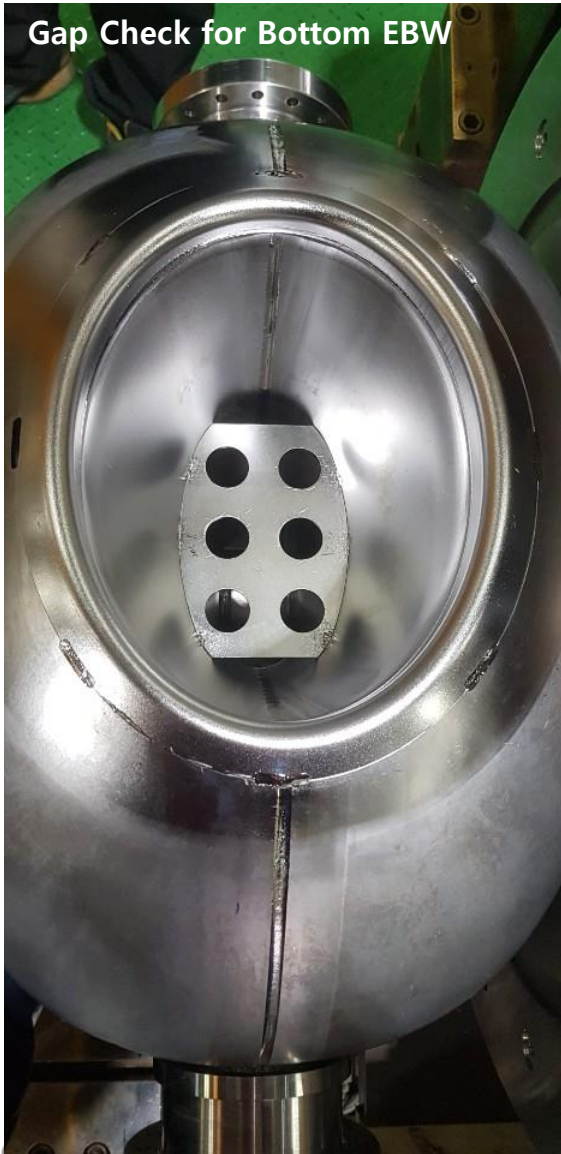
Chipping for Slight Gap Filling
