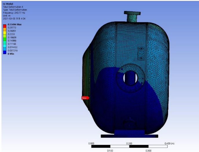
SSR1 ANSYS R18.0 Free Cover Fluctuation (240.77Hz)
