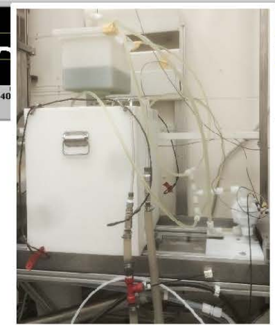
Bulk BCP of bare cavity
