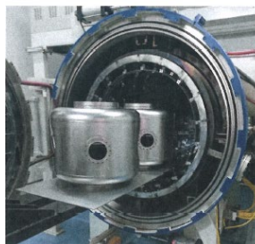
HTB: 3 hours at 800°C, 200°C/hour, 1e-3 Pa during HTB
