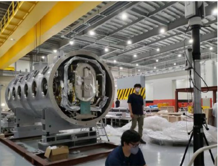
Insertion of cavity string into vacuum chamber
