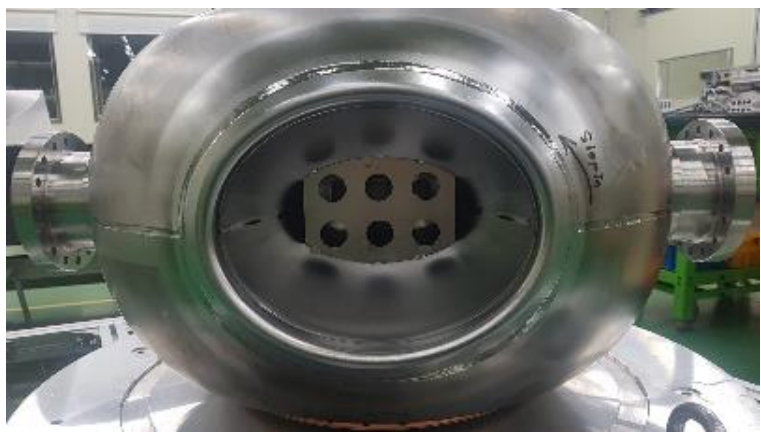
Bare Cavity : EBW (Check Welding Bead _ inside / outside)
