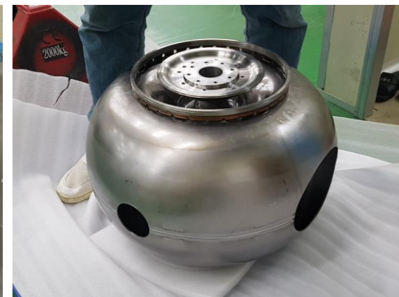
Half Shell + Half shell : EBW, Machining
