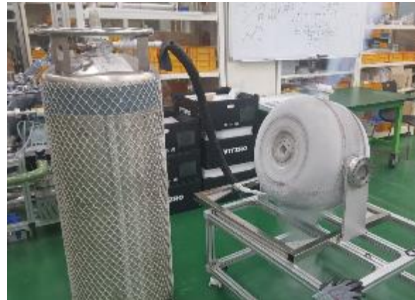
Simple Thermal Shock Test to check leakage
