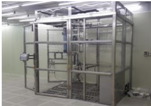
Cavity : HPR (Vertical, Horizontal, Tilted)
