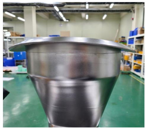
Collar + Spoke : EBW, Machining, CMM
