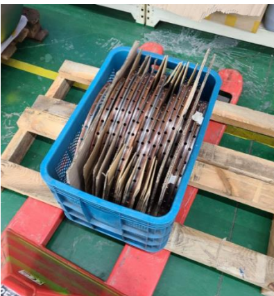
Stiffening Ring (Nb / Cu / STS) : TIG & EB welding
