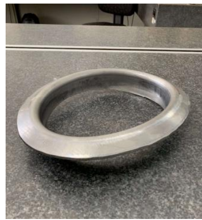
Collar + Spoke : EBW, Machining, CMM
