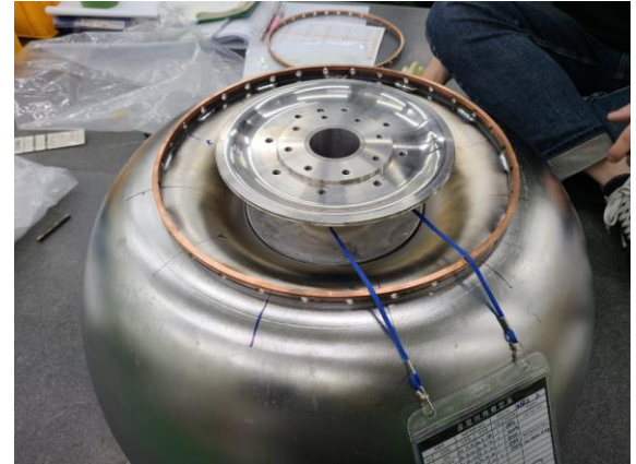
Half shell + Beam Port + stiffening ring : EBW
