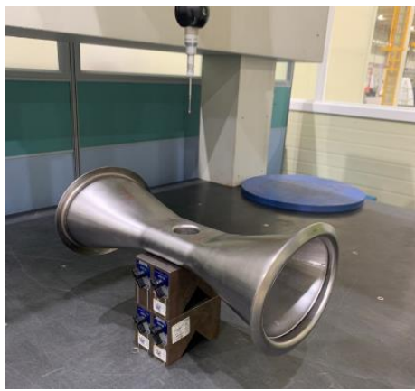
Collar + Spoke : EBW, Machining, CMM
