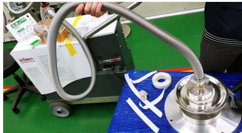
He Leak Test
