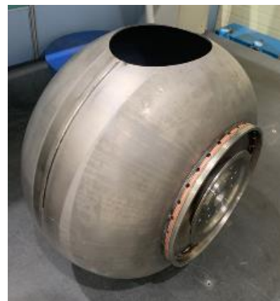
Half Shell + Half shell : EBW, Machining
