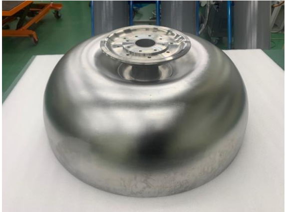
Half shell + Beam Port + stiffening ring : EBW
