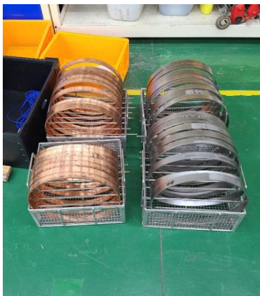
Stiffening Ring (Nb / Cu / STS) : TIG & EB welding
