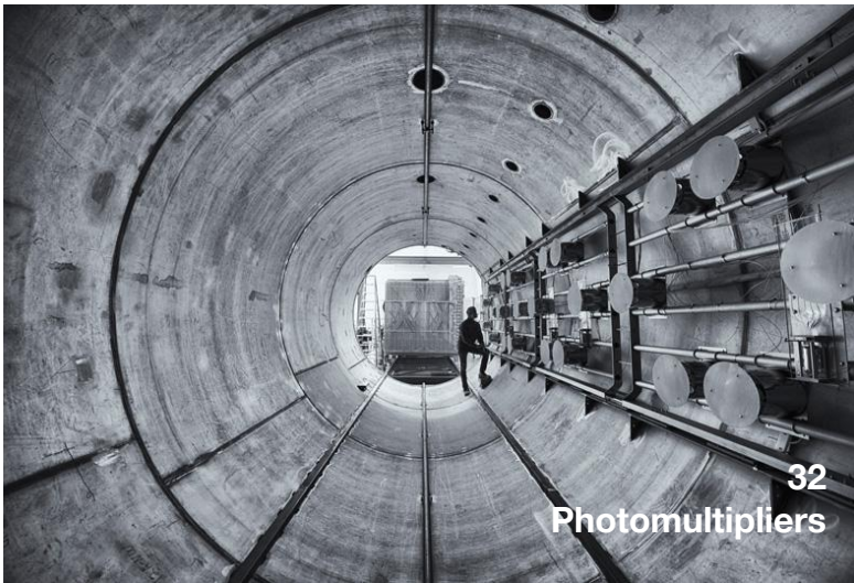
Inside the MicroBooNE LArTPC: 3 wire planes (8192 gold-coated wires)
