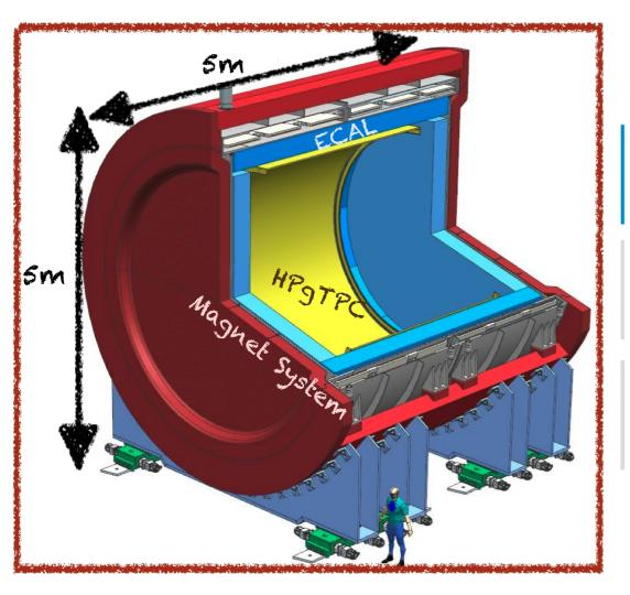
28. ECal for the gaseous argon detector
