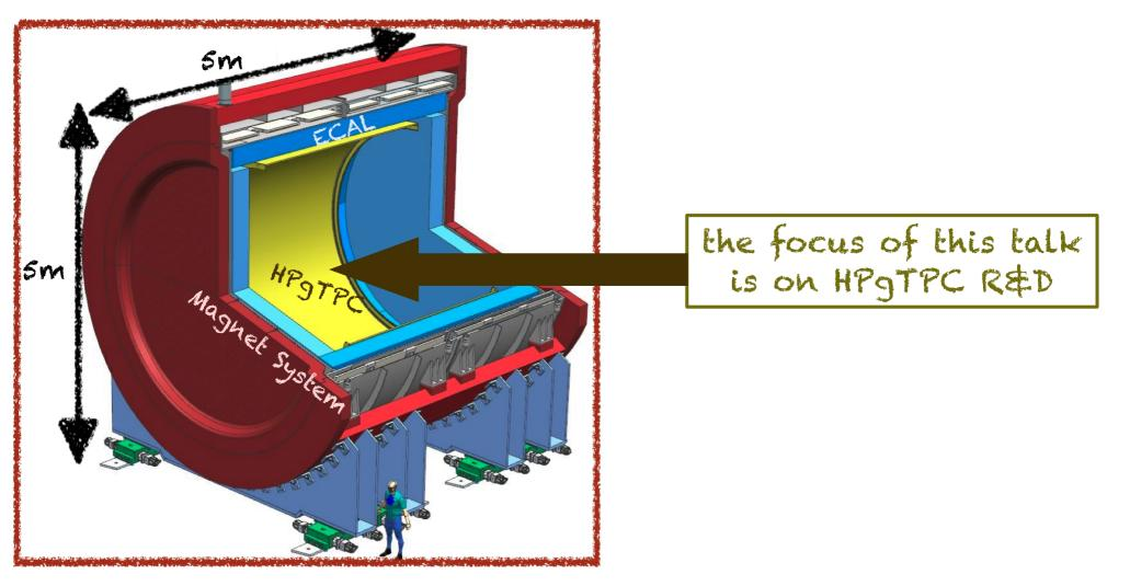
DUNE ND-GAr (formerly multi-purpose detector & sometimes the More Capable Near Detector Near Detector):
