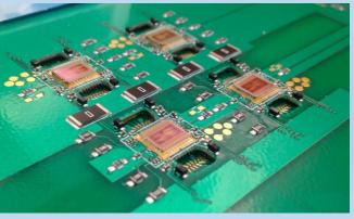
SAMPA chip developed for ALICE TPC upgrade and sPHENIX
