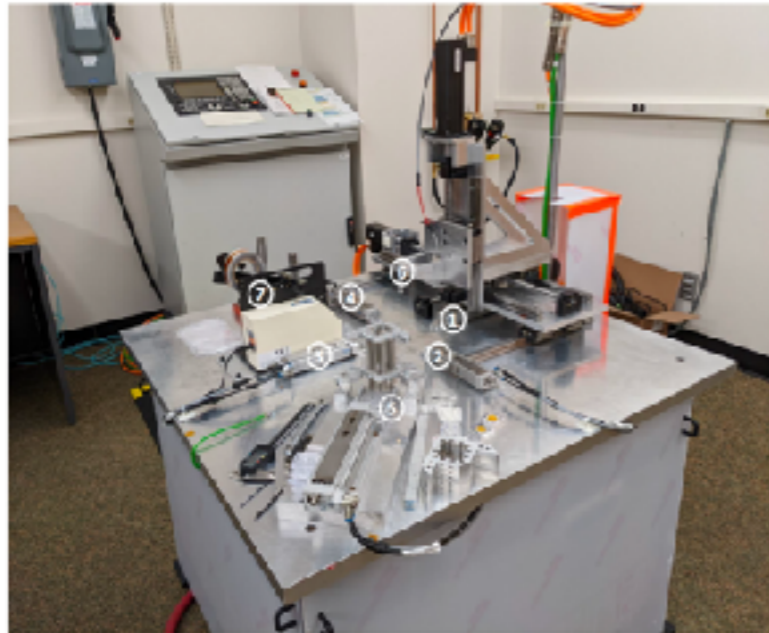
Figure 5.7: Automated scintillator tile wrapper overview. Shows in picture with labels are, 1-4: Actuator arms for folding the cut ESR flaps over the tiles, 5: Tile magazine and dispenser assembly, 6: z-axis (vertical up/down) end-effector with vacuum suction, 7: Kapton sticker dispenser.
