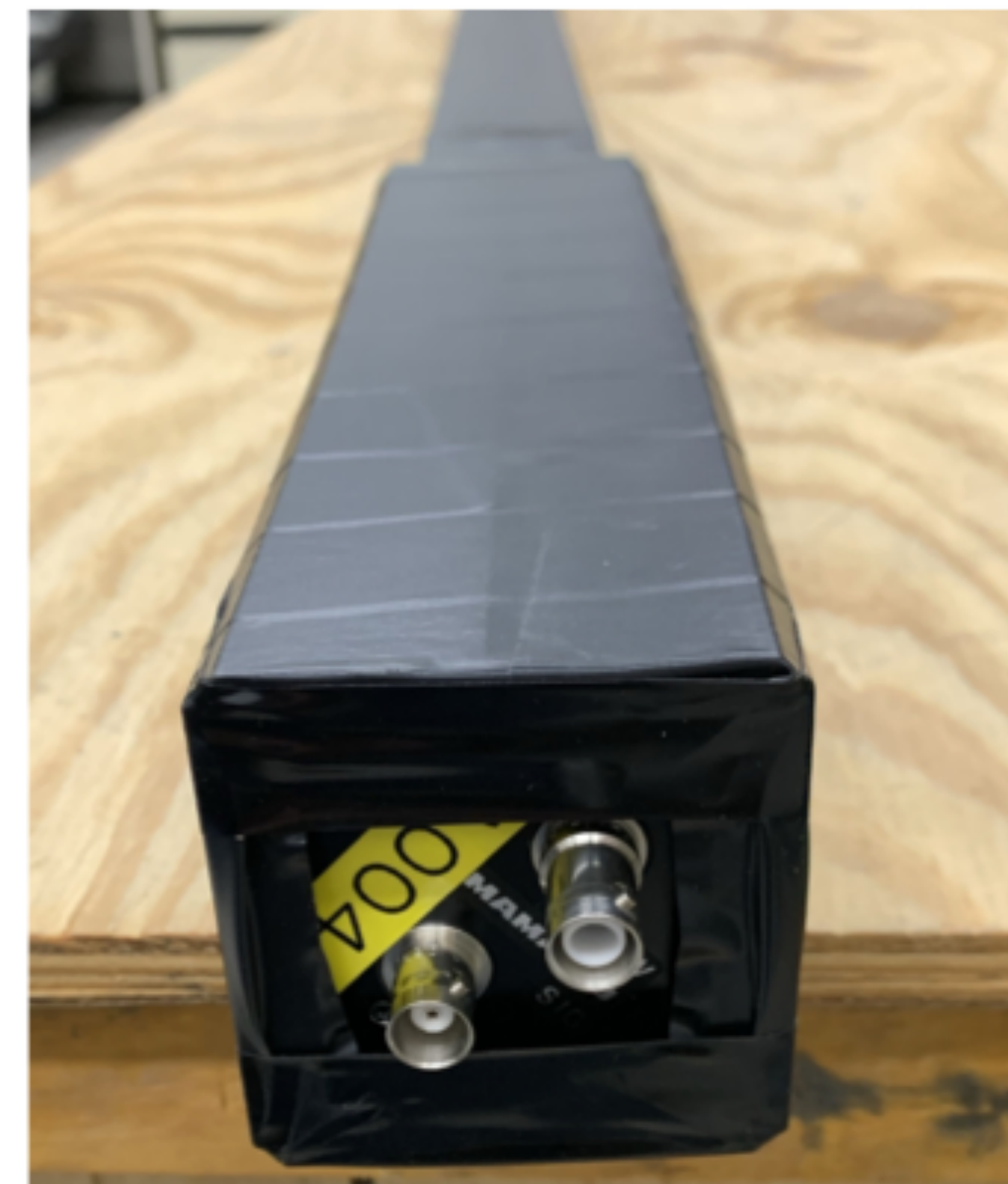
PMT support for coupling between PMT and scintillator
