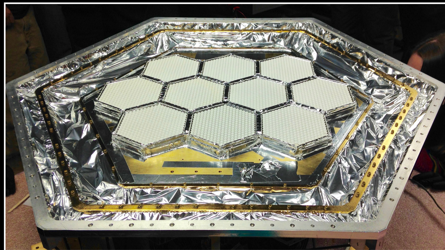
15,000 detectors at 95, 150, 220 GHz w/polarization
