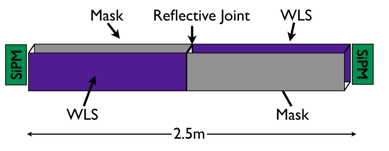
Readout from both ends of the bar. Each end sees photons from a different side of the APA.
