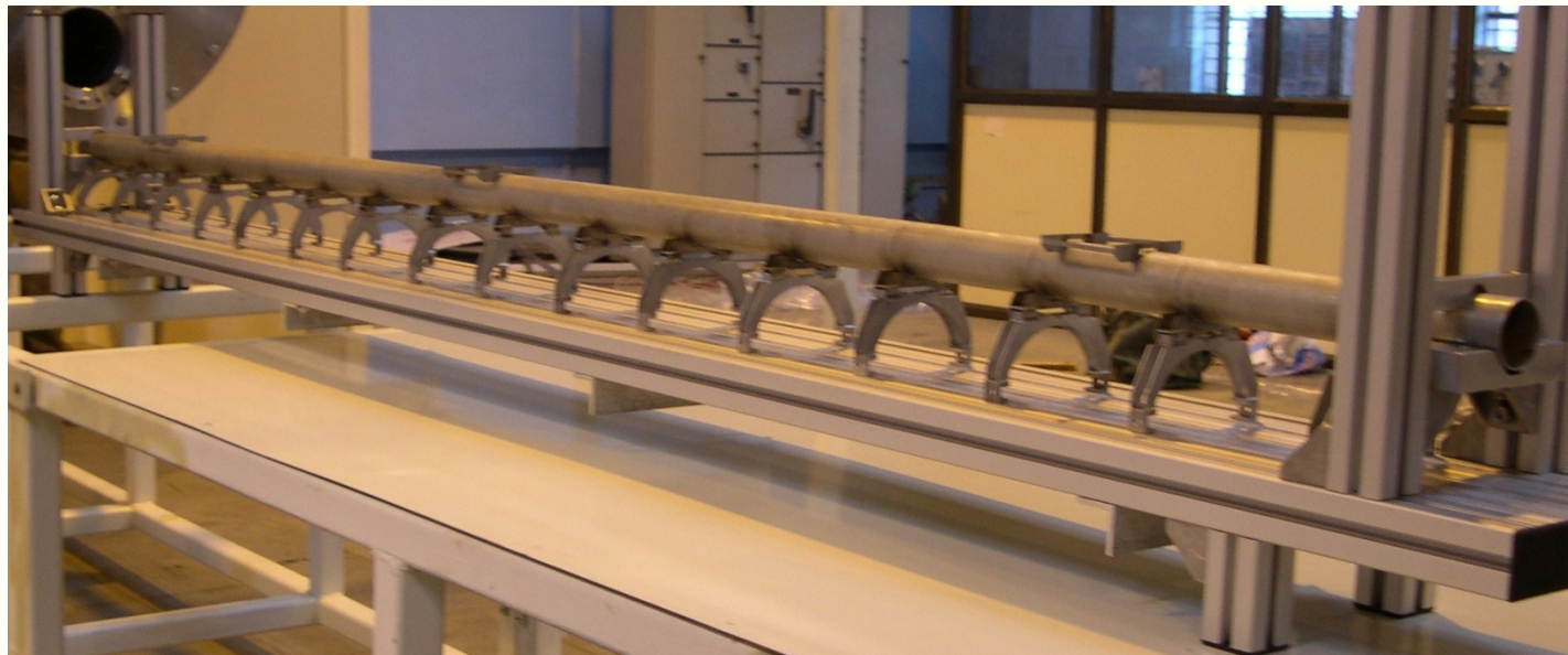
Laser welded prototype of the cavity support system
