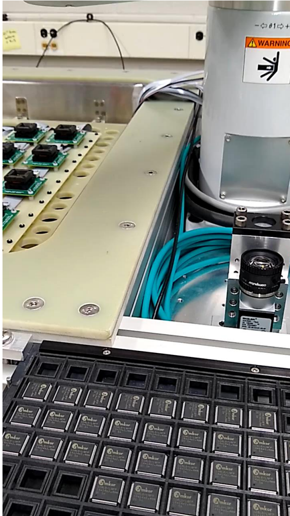
A timelapse of the RTS swapping a batch of 8 chips in the sockets in the current prototype setup
