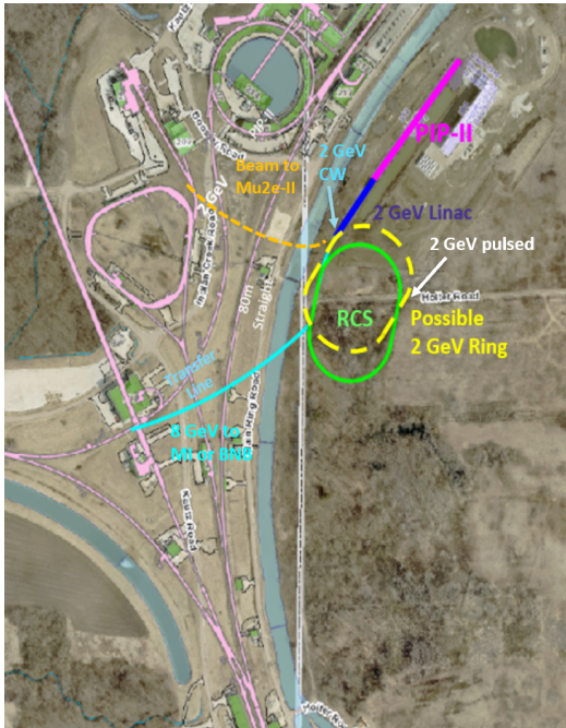
(a) Potential siting of ACE RCS configuration. The Tevatron field can accommodate other ARs or beamlines to operate alongside the 2-GeV Linac and 8-GeV RCS.
