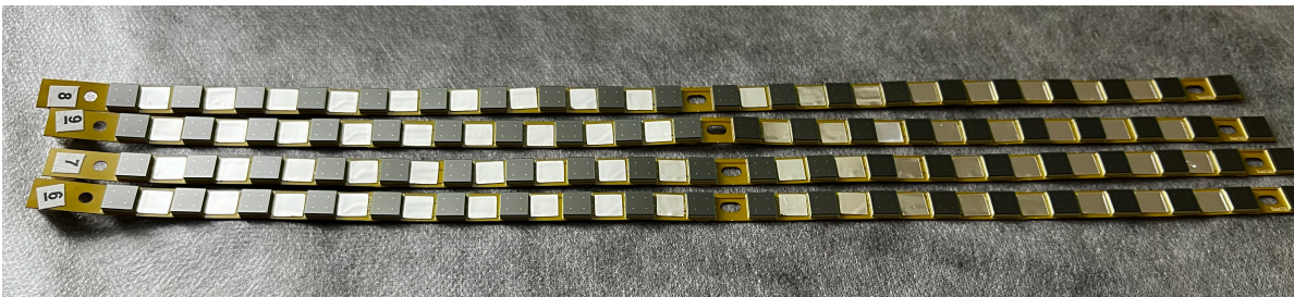
Hamamatsu MPPC S14160-6050HS [ V_{BD} = 32 \text{ V} at LAr T]
