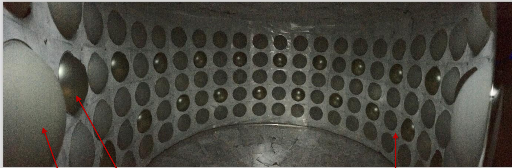
TPB coated reflector foils. Maximize light output to detect coherent neutrino-nucleus scattering
