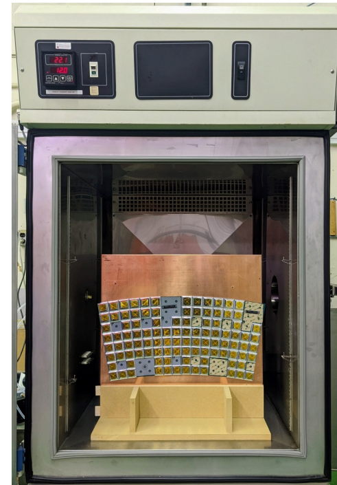
Thermal cycling trial in the oven
