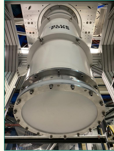
Cryostat window + IR filter for optical testing
