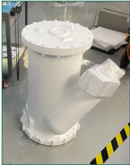
SPT-SLIM cryostat test installation
