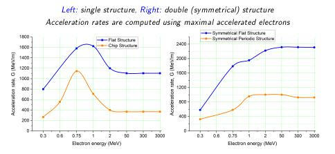
Note the acceleration rate don't depend from beam energy for ultra-relativistic electrons (???) both for single and double DLA.
